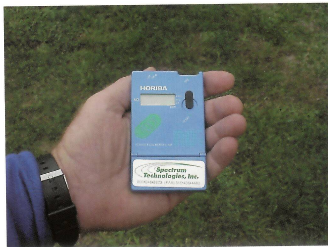
Hand-held nitrate meters are used to measure soil nitrate levels in the field and can be a useful tool when deciding how much nitrogen fertilizer to apply.
