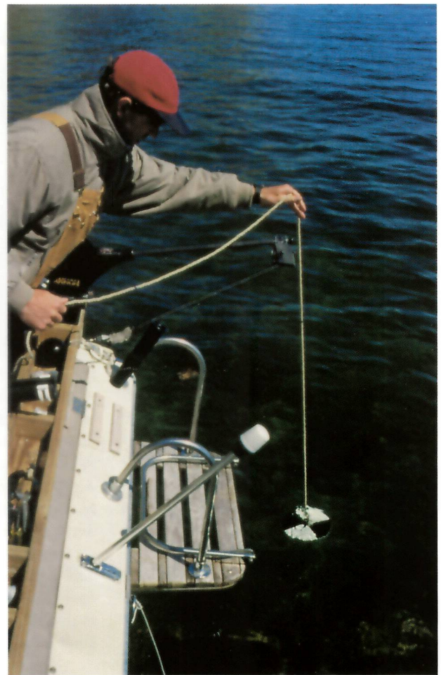
Water clarity is measured by lowering the black and white painted disc (Secchi disc) into the water and determining the depth at which it can no longer be seen.
